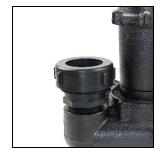
**1.** Insert the Quick-Connect fitting into the pump discharge outlet and tighten.
